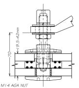
M I 4 SPRING WASHER 35 x 2 x M | 4 FLAT WASHER 35 x 0.8 x M | 4 FIBRE GASKET 445 SPIDER PALM 35 x O.8 x M I 4 FIBRE GASKET 35 x 2 x M I 4 FLAT WASHER MI4 NUT MITH NOT 60/22/42n SPIDER FITTING, INCLUDES BUSH TO SUIT GLASS THICKNESS IGU SPACER - 60 x 1/2mm DISC/60 x 1/2" DISC
