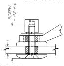
MIO AGA NUT MIO AGA NUI MIO SPRING WASHER 30 × 2 × MIO FLAT WASHER 30 × 0.8 × MIO FIBRE GASKET 14.5 × 10.5 × 9.5 BUSH FOR SPIDER PALM 445 SPIDER PALM 50 x 6mm DISC 50 x 10.5 x 0.8 FIBRE GASKET 19.5 x 10.5 BUSH, TO SUIT GLASS THICKNESS 50 x 10.5 x 0.8 FIBRE GASKET 50 x 6 x M I O RA DISC
