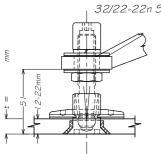
M I 4 AGA NUT M I 4 SPRING WASHER 35 x 2 x M | 4 FLAT WASHER 35 x 0.8 x M | 4 FIBRE GASKET 445 SPIDER PALM 35 x 0.8 x M I 4 FIBRE GASKET 35 x 2 x M | 4 FLAT WASHER M | 4 NUT 32/22/22n SPIDER FITTING, INCLUDES BUSH TO SUIT GLASS THICKNESS
