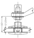
M I 4 AGA NUT M I 4 SPRING WASHER 35 x 2 x M | 4 FLAT WASHER 35 x 0.8 x M | 4 FIBRE GASKET 445 SPIDER PALM 35 x O.8 x M I 4 FIBRE GASKET 35 x 2 x M | 4 FLAT WASHER M | 4 NUT 60/22/22n SPIDER FITTING, INCLUDES BUSH TO SUIT GLASS THICKNESS
