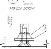
M8 AGA NUT M8 SPRING WASHER 20 x 2 x M8 FLAT WASHER 20 x 0.8 x M8 FIBRE GASKET 444 SPIDER PALM 35 x 0.8 x M8 FIBRE GASKET M8 CSK BUSH, TO SUIT GLASS THICKNESS
