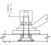
MIO AGA NUT MIO SPRING WASHER 20 x 2 x MIO FLAT WASHER 20 x 0.8 x MIO FIBRE GASKET 444 SPIDER PALM 50 x Gmm DISC 50 x 10.5 x 0.8 FIBRE GASKET M10 CSK BUSH, TO SUIT GLASS THICKNESS
